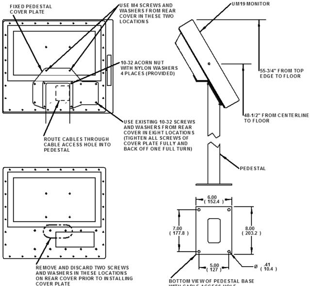
BOTTOM VIEW OF PEDESTAL BASE WITH CABLE ACCESS HOLE
